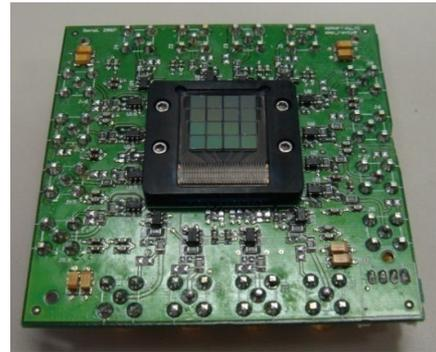
Fig.2 Photograph of the SPMArray and preamplifier board
