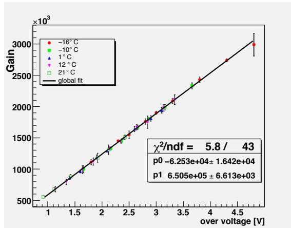
Fig. 4. Gain dependance vs. the over voltage.
