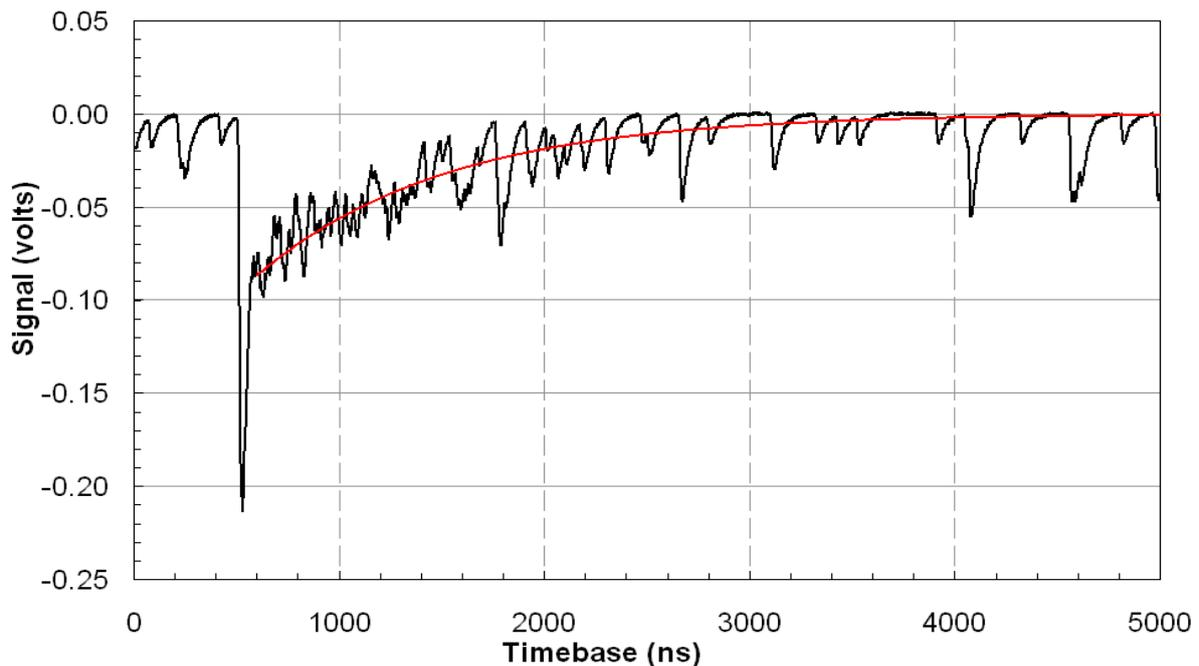
Figure 10. Secondary scintillation spectrum from Fe-55 in a liquid argon system. (SiPM over-voltage=1V,  $V_{TGEM} = 9.91KV$ , Drift field in liquid = 2.5KV/cm, 5.9KeV peak corresponding to 62 photoelectrons, 1037508 total events.)
