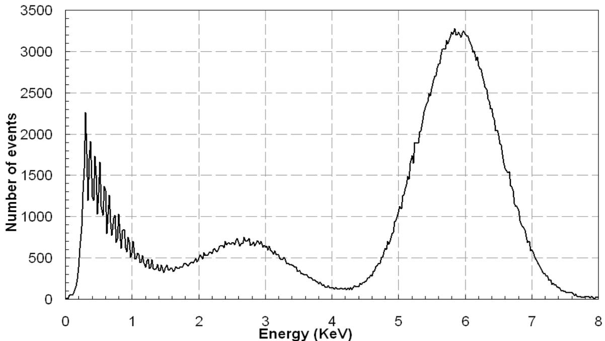
Figure 7. Secondary scintillation in 1 bar  $-189^{\circ}\text{C}$  gaseous argon as a function of the voltage across a TGEM due to the passage of charge generated via the interaction of an Fe-55 source in the liquid phase within a  $2.5\text{KV/cm}$  drift field.
