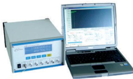
A single-photon detector module for the near infrared, the id201, is available from **id Quantique** (Carouge, Switzerland). The system is based on a cooled InGaAs/InP APD operating in Geiger mode, and covers the wavelength range of 900–1,700 nm. It offers a detection probability of up to 25% at 1,550 nm. Signal-to-noise performance is optimized by setting the operating temperature at –50 °C with a thermoelectric cooler, which has a temperature variation of less than 0.1 °C.
