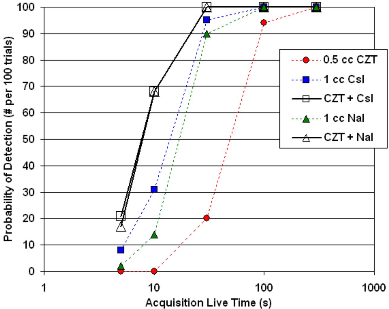
Figure 4. Results of identification testing with a  $100 \mu\text{R/h } ^{137}\text{Cs}$  source, with each data point generated by 100 trial acquisitions. Trial acquisition times were for 5, 10, 30, 100, and 300 seconds. Lines added to guide the eye
