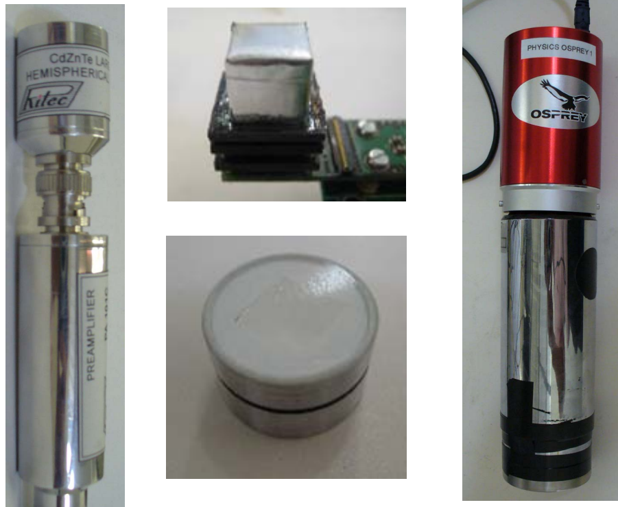
Figure 2. Component detectors used for the evaluations. The 0.5 cm 3 CZT (Ritec CZT/500, left), the 1 cm 3 CsI (Scionix) mounted on the silicon photomultiplier prior to final light-tight wrapping (SensL SPMArray4, upper middle), the 1 cm 3 NaI (Scionix, bottom middle), and NaI mounted on a photomultiplier tube and Canberra Osprey MCA (right).
