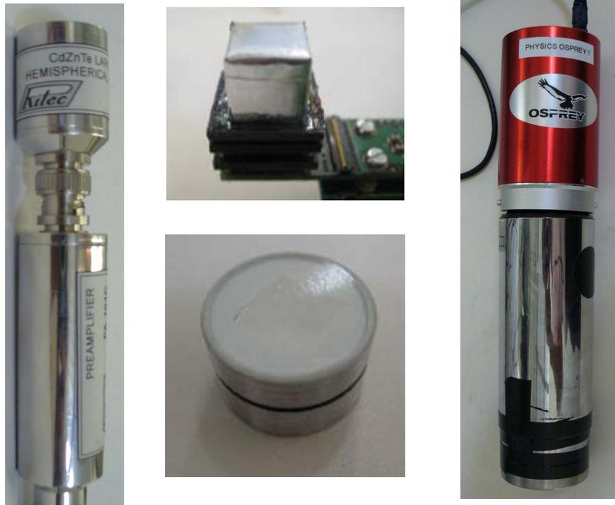
Figure 2. Component detectors used for the evaluations. The 0.5 cm<sup>3</sup> CZT (Ritec CZT/500, left), the 1 cm<sup>3</sup> CsI (Scionix) mounted on the silicon photomultiplier prior to final light-tight wrapping (SensL SPMArray4, upper middle), the 1 cm<sup>3</sup> NaI (Scionix, bottom middle), and NaI mounted on a photomultiplier tube and Canberra Osprey MCA (right).
