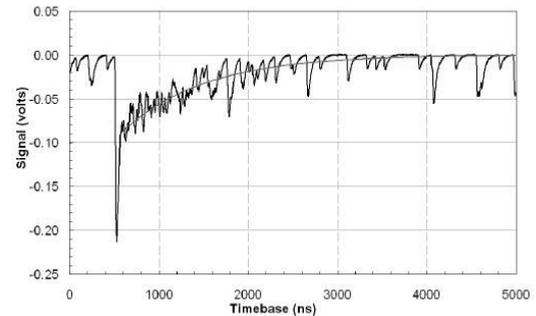
Figure 3. Secondary scintillation light pulse produced by Fe55 source in LAr system.
