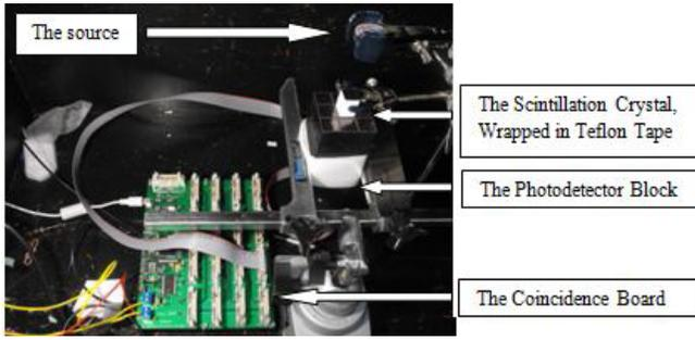
Fig. 2. The experiment setup for energy resolution and uniformity analysis, showing the detector block connected to the coincidence board, the  $^{22}\text{Na}$  source and the LYSO crystal array wrapped in Teflon.
