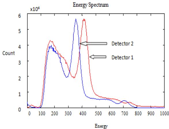
Fig. 3. The global energy spectrum of detectors 1 and 2 with the 511 keV photopeak energy resolutions of  $19.0 \pm 2.5\%$  and  $18.1 \pm 5.0\%$  FWHM, respectively. The global energy spectrum of each detector block was calculated by adjusting (in post-processing) the individual energy spectra of its pixels to have the same photopeak mean value.
