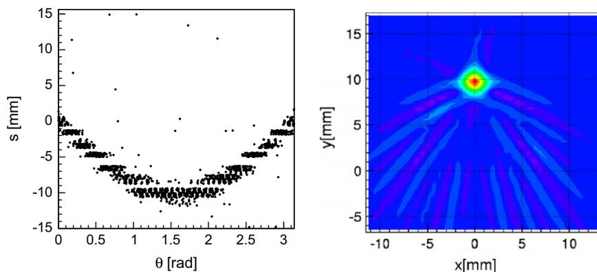
Fig. 2. Sinogram (left) and reconstructed image (right) resulting from the simulation of the response of the PET system based on LySO/SiPM detectors to a  $^{18}\text{F}$  source of 0.2 mm radius placed at a vertical distance of 1 cm from the centre of the tomograph.
