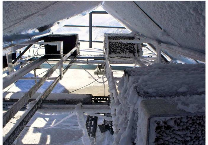
**Fig. 1:** Prototype detector installed at Sphinx (HFSJG) to test upward/downward particles separation and environmental effects.
